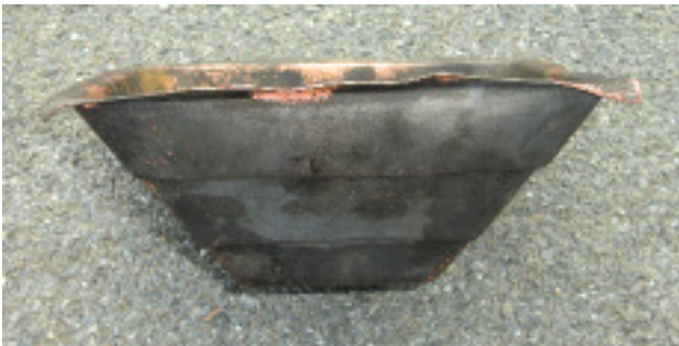
Above and below: Warped pyramids that need re-pressing. Below right, a repaired pyramid.
